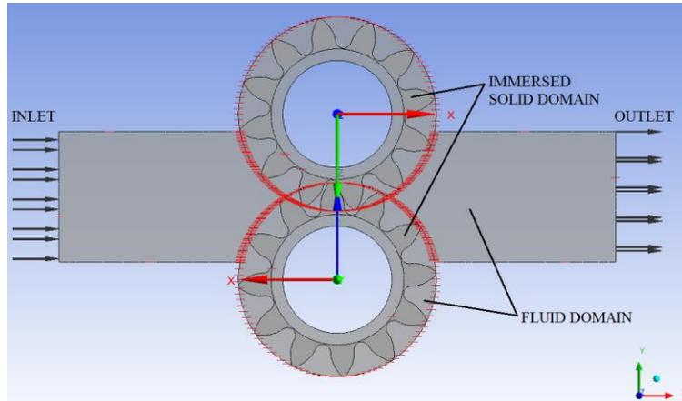
Fig. 2. Simplified 2D model of a PGP620 pump
