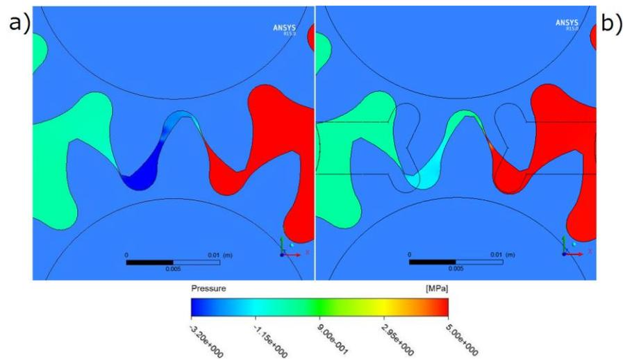
**Fig. 10.** Pressure contours for geometry a) without relief grooves, b) with relief grooves ( $p=5$  MPa,  $n= 2000$  rev/min)- trapped volume is increasing
