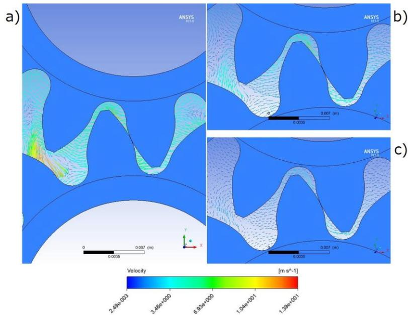
**Fig. 4.** Velocity vectors for different rotational speeds a) 2000 rev/min, b) 1000 rev/min, c) 500 rev/min
