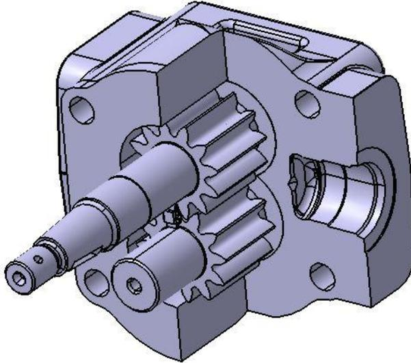
**Fig. 1.** 3D geometry model of an external gear pump created via CATIA V5
