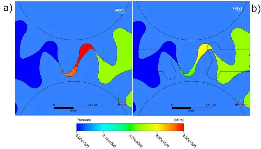
**Fig. 9.** Pressure contours for geometry a) without relief grooves, b) with relief grooves ( $p=5$  MPa,  $n= 2000$  rev/min)- trapped volume is decreasing
