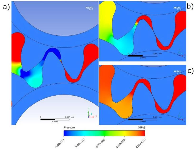
**Fig. 5.** Pressure distribution for different rotational speeds a) 2000rev/min, b) 1000 rev/min, c) 500 rev/min
