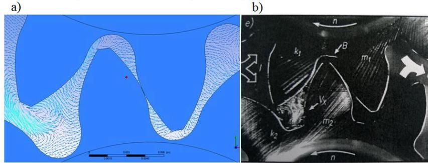
**Fig. 3.** Comparison of a) simulation research, b) visualization research
