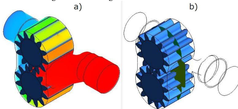
Fig. 8. Pressure distribution a) volume b) cutting plane
