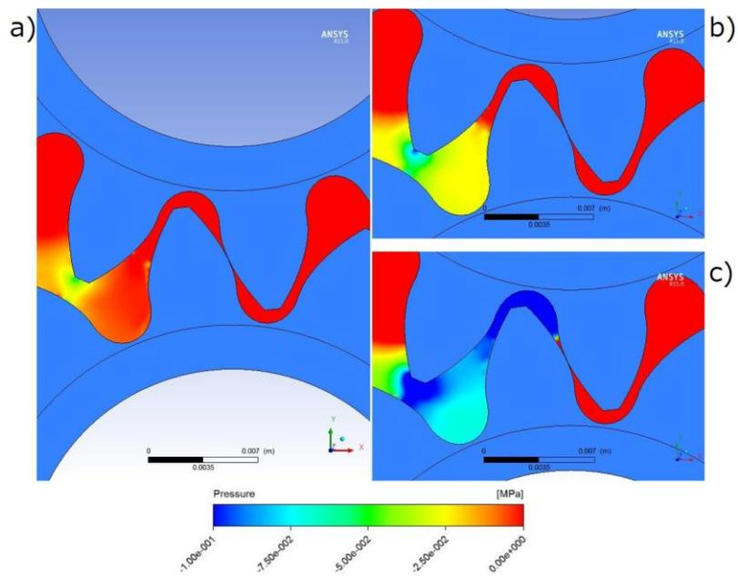
**Fig. 7.** Pressure distribution for different values of discharge pressure a) 15 MPa, b) 10 MPa, c) 5 MPa
