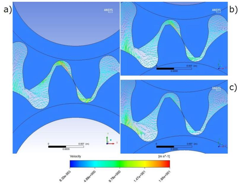
**Fig. 6.** Velocity vectors for different values of discharge pressure a) 15 MPa, b) 10 MPa, c) 5 MPa
