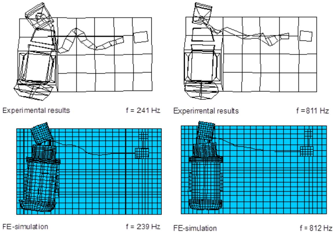
Figure 8: Comparison of experimental and simulation results.
