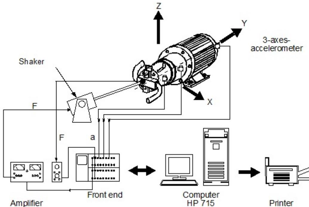
Figure 5: Measurement setup for Experimental Modal Analysis (EMA).
