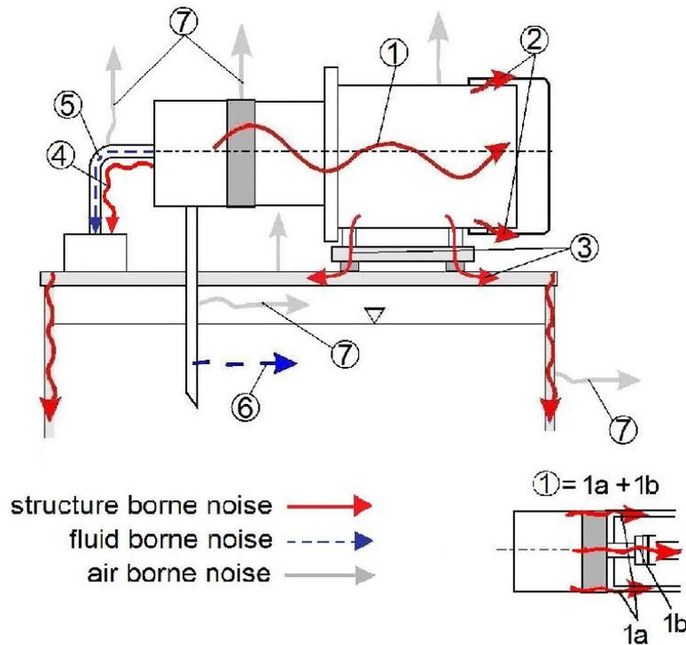
Figure 1: Noise transmission paths in fluid power unit.
