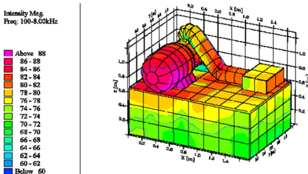
Figure 3:Sound intensity distribution on the surface of the power unit ( $p=10$  MPa), frequency range: 100 Hz -8 000 Hz.
