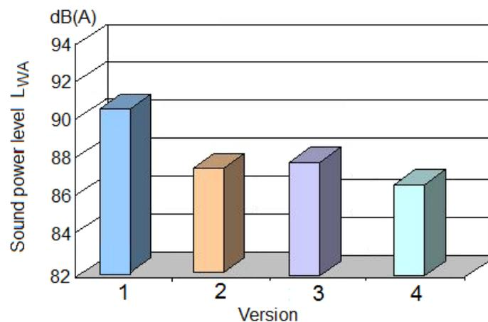
Figure 10: Comparison of sound power levels of power unit with vibration measures according Fig. 8.
