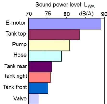
Figure 4: Ranking of noise sources in the power unit ( $Q=63\text{l/min}$ ,  $p = 10\text{ MPa}$ ).
