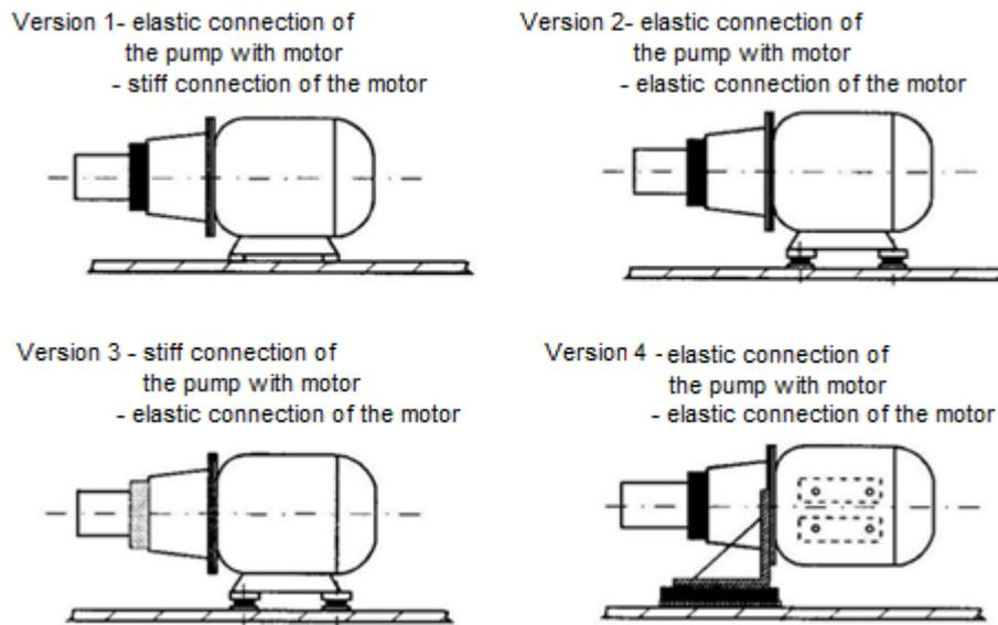
Figure 9: Investigated modifications of the pump motor group.
