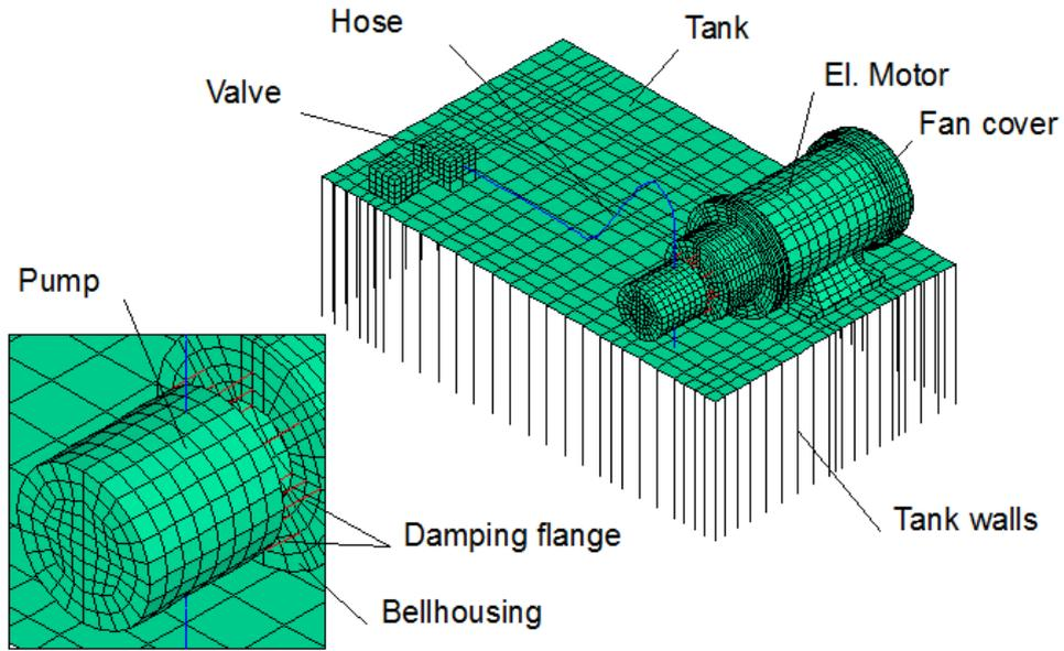
Figure 7: FE- Model of the power unit.
