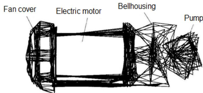
Figure 6: Operational Deflection Shape Analysis at 1205 Hz for the pump motor group ( $p = 25$  MPa).
